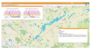
Figure 1: Global Flood Monitoring (GFM) products shown on the EFAS map viewer
